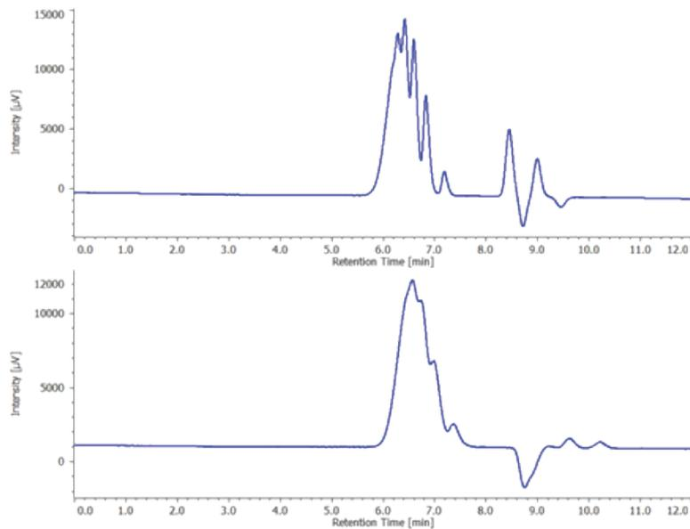
**Figure 1.** Chromatogram of polystyrene oligomer Top: RI-4035, Bottom: RI-2031
