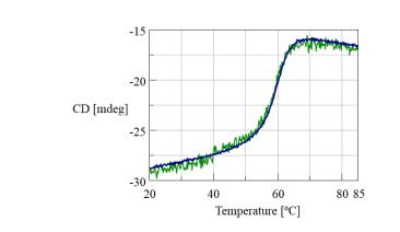
Figure 2. Thermal denaturation curve of ribonuclease A measured at a wavelength of 222 nm. The green curve was obtained using the capillary cell while the blue curve was measured using the 1 mm rectangular cell.
